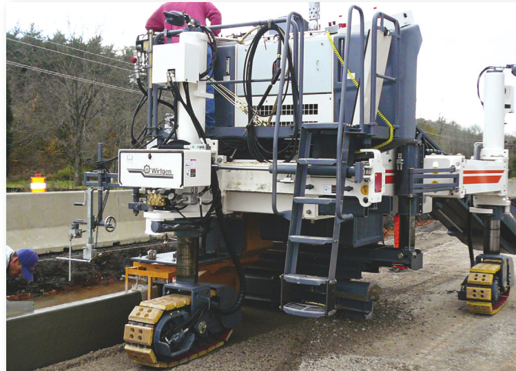
Wirtgen's 27,500-pound, three-track SP15 will telescope molds 28 inches to either its left or right side.
