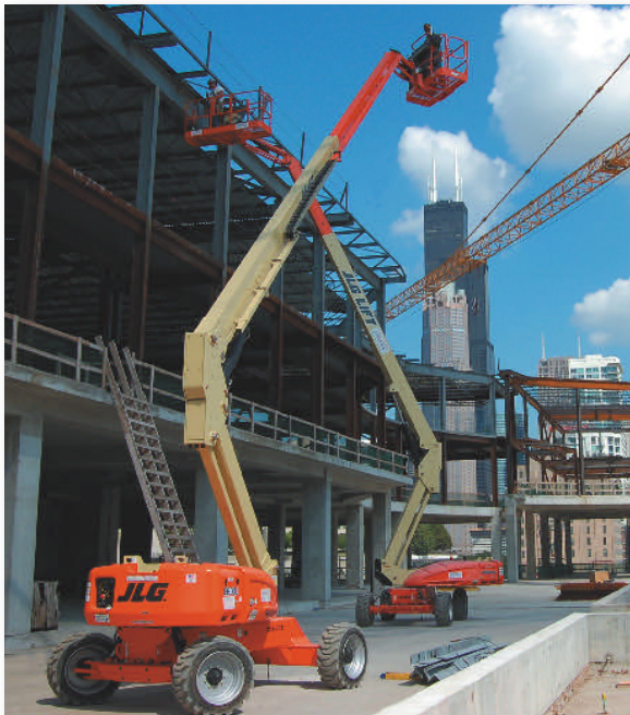
JLG E600 articulating aerial work platform is electric drive, so diesel emissions are eliminated. The site also benefits from the unit's low noise emissions.
