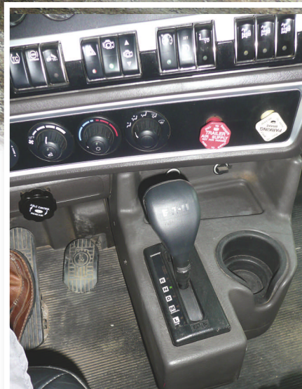
Dump truck had a paddle-style shift selector, which can be operated by feel; tranny will also work with a keypad type. Either way, it's usually best to put it in D-for-drive and leave it alone.
