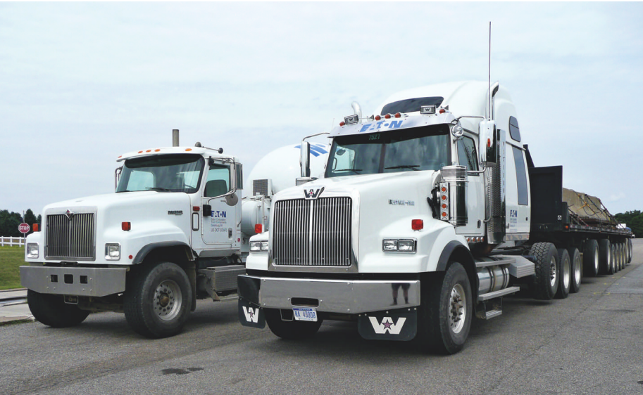
International PayStar mixer had a 9-speed UltraShift Plus and the Western Star 4900 tractor had an 18-speed version. Three vocational models have high ratio coverage and torque capacities of 1,450 to 2,250 pounds-feet.
